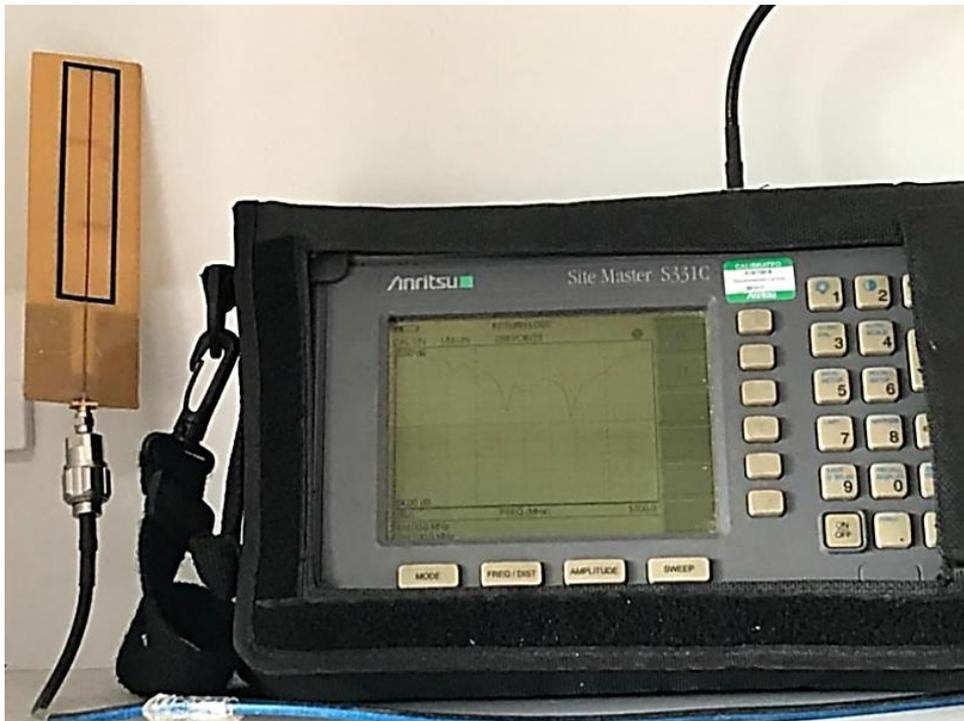
Fig. 4. The return loss measurement setup.
