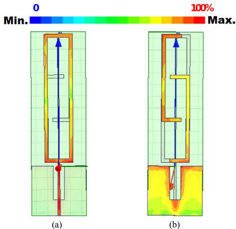
Fig. 7. Normalized current density distributions at: (a) 700 MHz and (b) 990 MHz.
