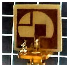
Fig.8. Fabricated prototype of the proposed antenna.
