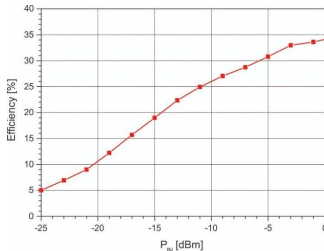
Fig. 9. Measured RF rectifier efficiency as a function of  $P_{IN}$  at 2.45 GHz.
