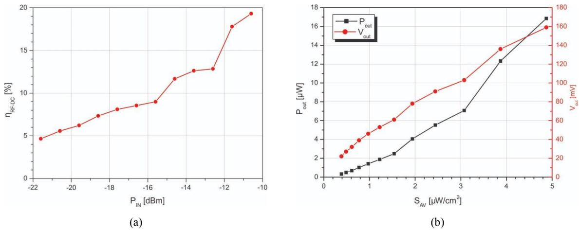
Fig. 11. Rectenna parameters: (a) conversion efficiency and (b) output parameters.
