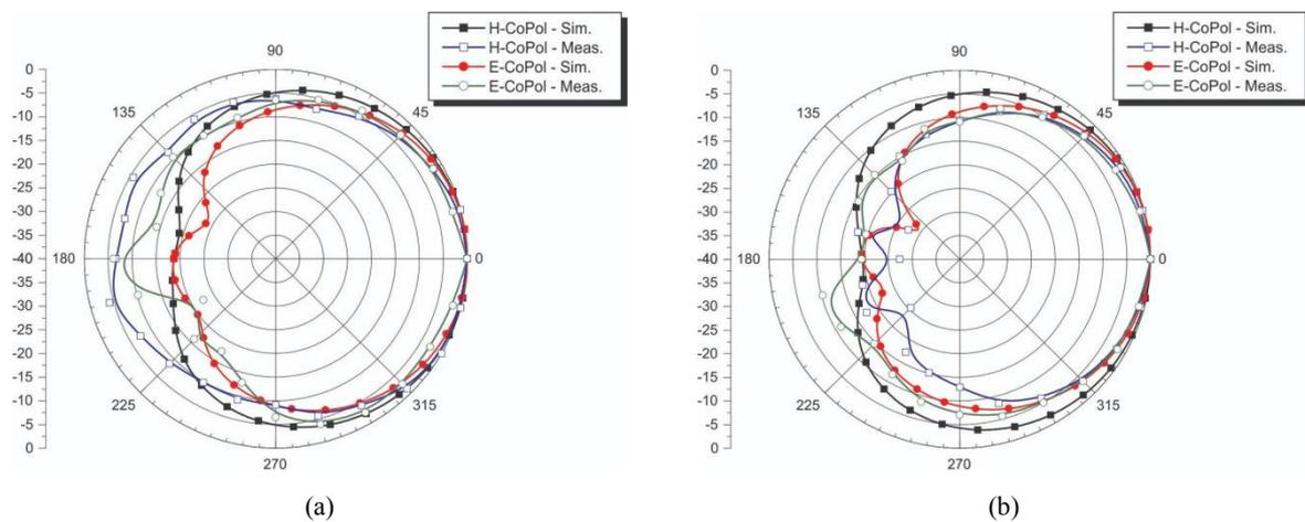
Fig. 6. Radiation pattern characteristics at (a) 1.8 GHz and (b) 2.45 GHz.
