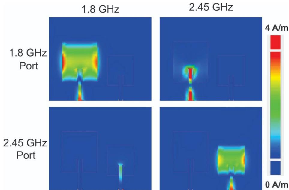
Fig. 3. Current density of DPA for RF sources applied to the port of 1.8 (top) and 2.45 GHz (bottom) at the frequencies of 1.8 (left) and 2.45 GHz (right).
