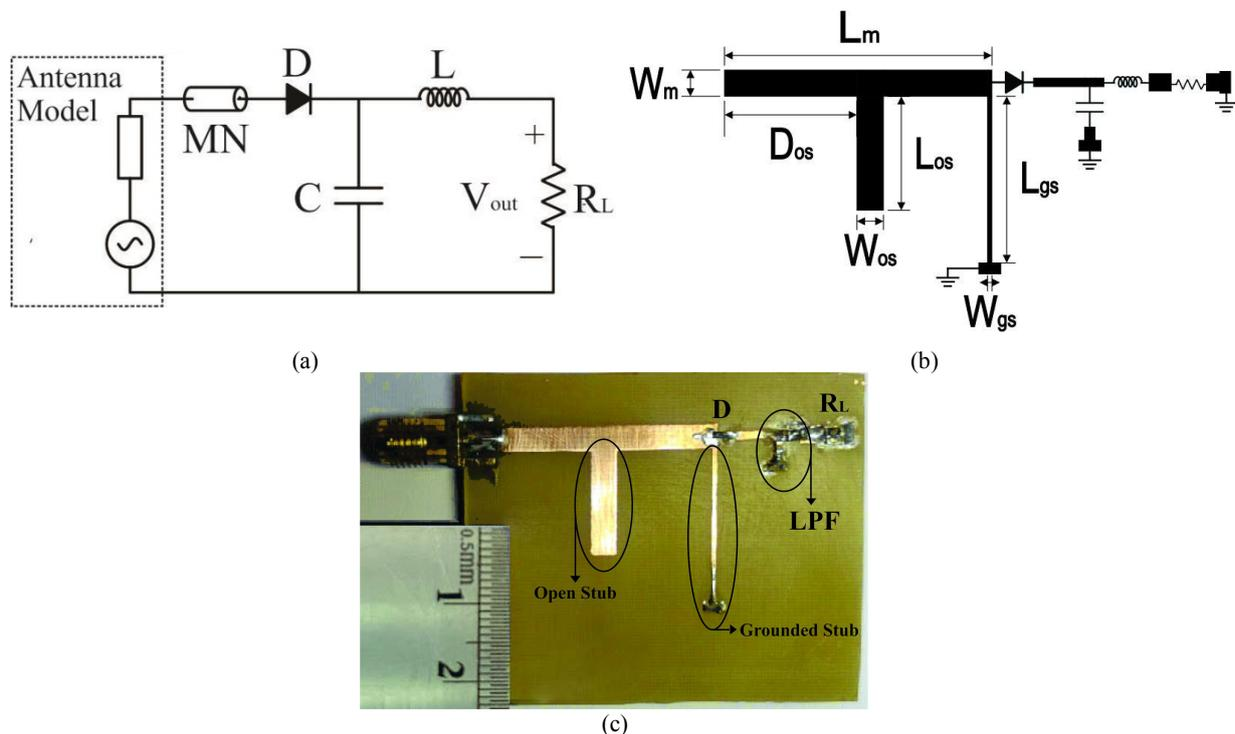
Fig. 7. The RF rectifier (a) schematic, (b) layout and (c) prototype.
