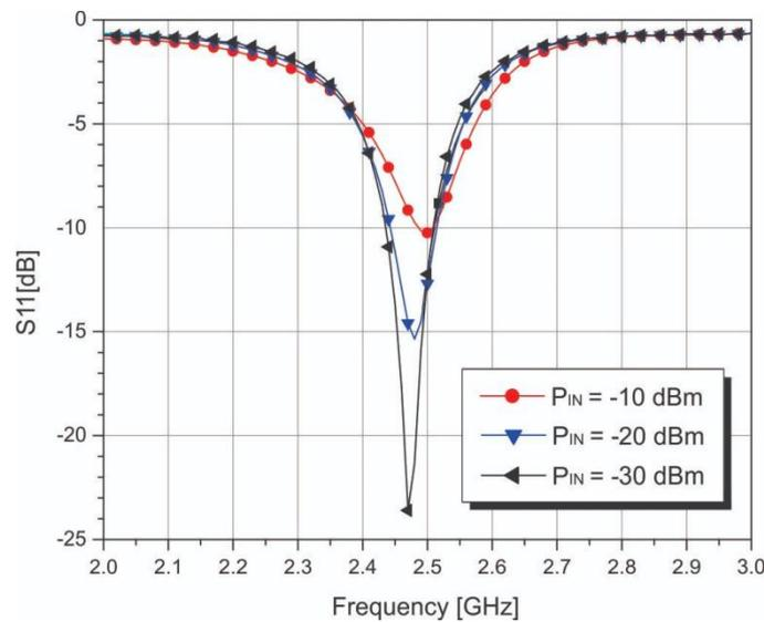
Fig. 8. Measured S11 parameter of the RF rectifier for  $P_{IN}$  from -30 to -10 dBm.
