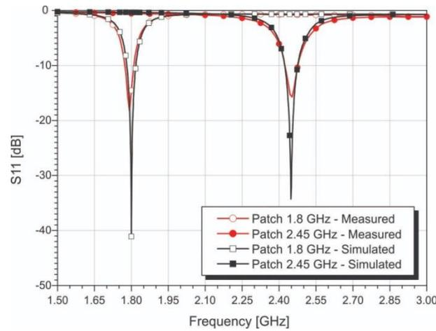
Fig. 5. Simulated and measured reflection coefficient of DPA.
