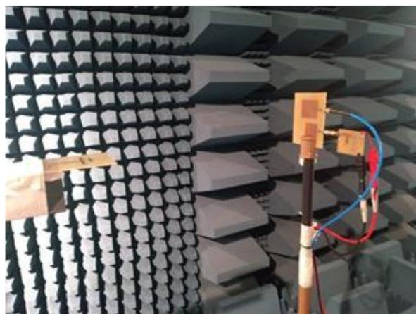
Fig. 10. Measurement setup for RFEH parameters.
