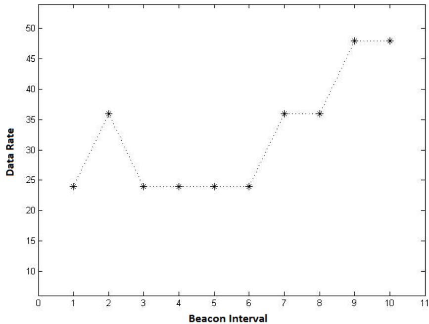
Fig. 4. Rate switching for various beacon intervals
