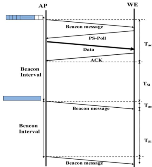
Fig. 3. Energy Efficient Rate Adaptation Algorithm along with PSM
