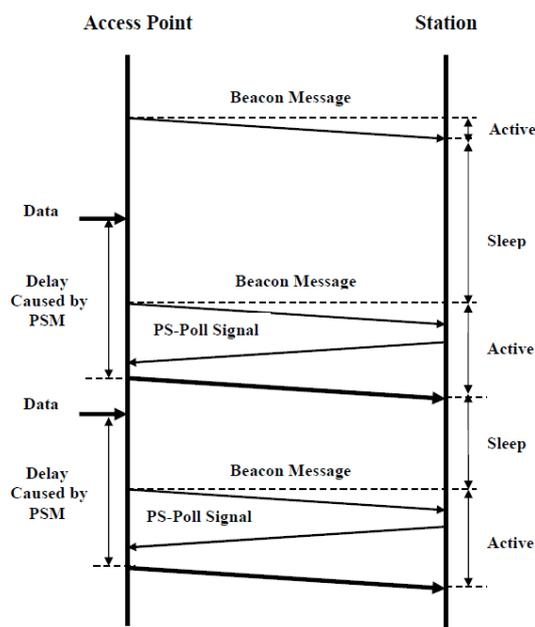
Fig. 2. Illustration of PSM for front end of FiWi network
