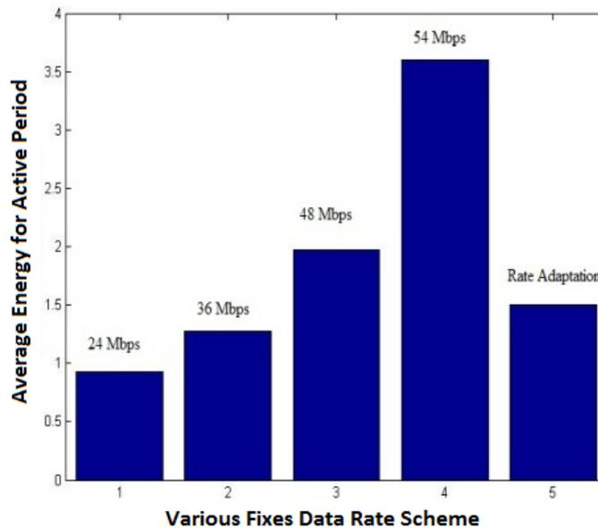
Fig.6. Average energy consumption during active state
