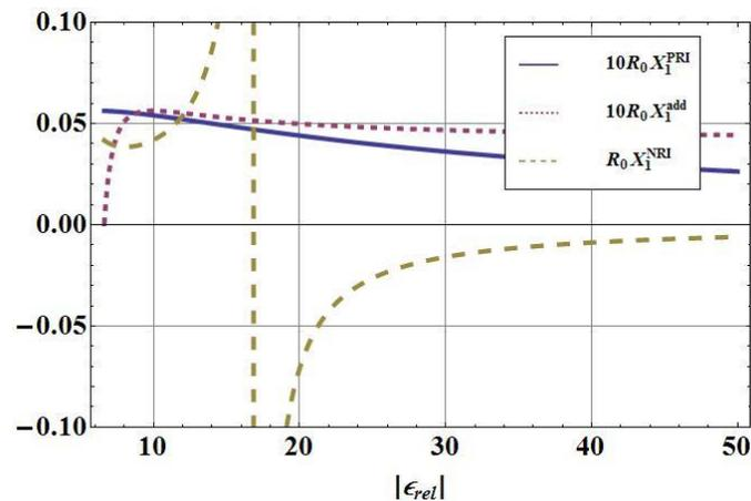
Fig. 3. First reactance  $X_1$  (NRI, PRI and *add*) for  $|\epsilon_{rel}| > 6.606$ . It represents the first lumped element of an equivalent RLC (admittance) circuit model. For visualization purposes, multiplicative factors are included for  $X_1^{PRI}$  and  $X_1^{add}$ .
