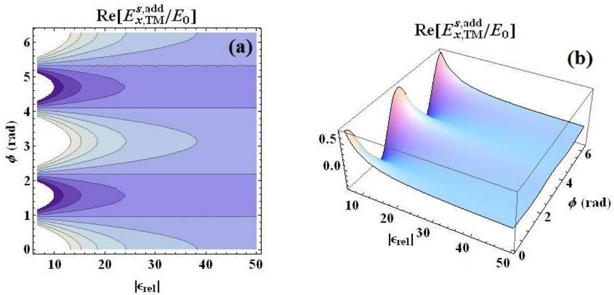
Fig. 1. Additional (pure metamaterial part of) TM  $E_x$ -field in the  $\theta = \pi/2$  plane and at  $r = 2a$  for a NRI sphere with  $ka = 0.01$ ,  $\mu_{rel} = -\mu_0$  under plane wave illumination. The wave propagates along  $+z$  and is  $x$ -polarized.
