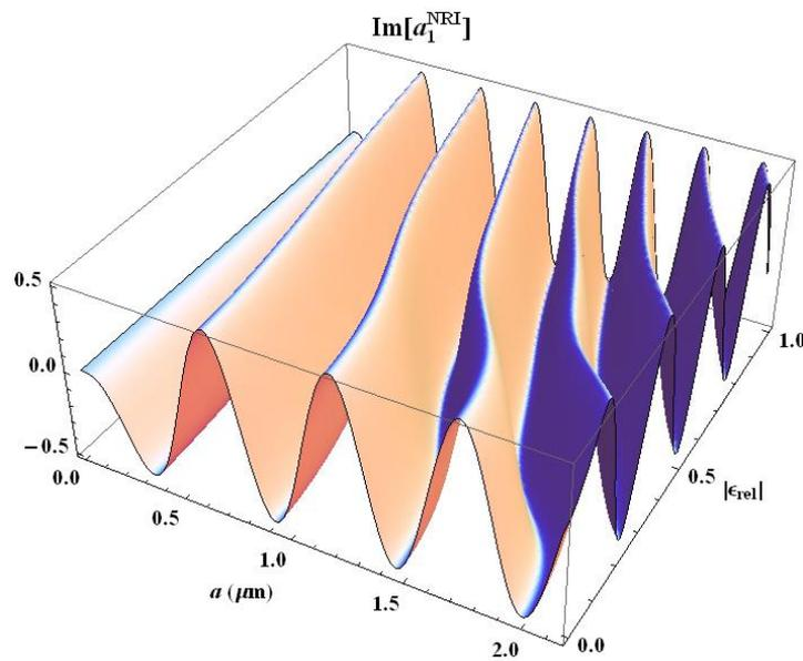
Fig. 6.  $a_1^{NRI}$  as function of  $\epsilon_{rel}$  and  $a$ .  $\lambda = 1064$  nm.
