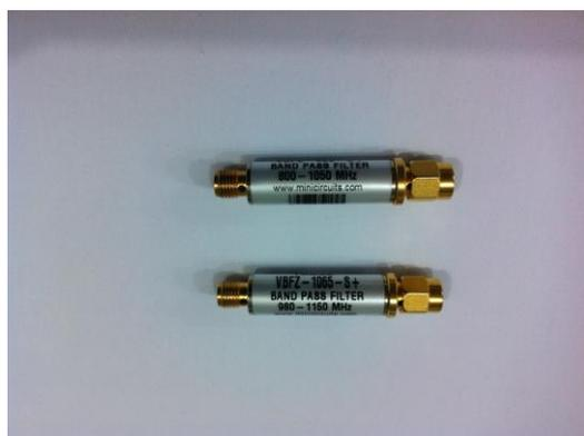
Fig. 6. 925MHz and 1065MHz filters used for testing.
