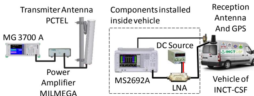
Fig. 3. Measurement Setup.
