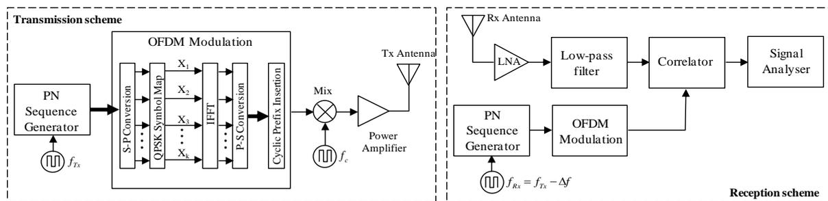
Fig. 1. Proposed Sounding Technique.
