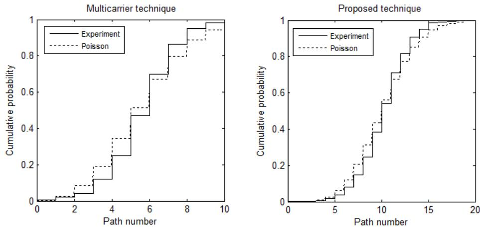
Fig. 8. Cumulative distribution function of number of multipath components.
