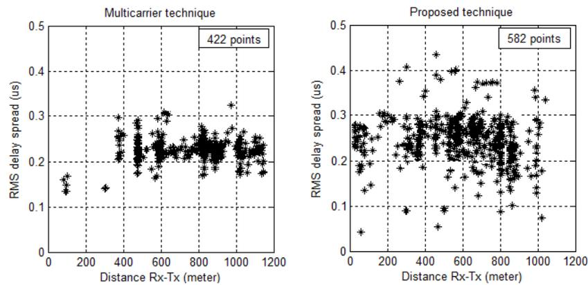
Fig. 6. Measured values of RMS delay spread.
