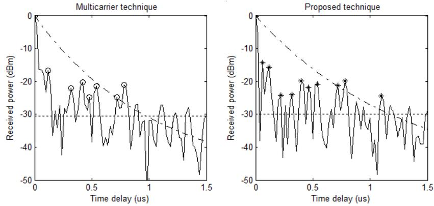
Fig. 5. Measured and CFAR filtered power delay profiles at a point: (a) Conventional multicarrier technique; (b) proposed technique.
