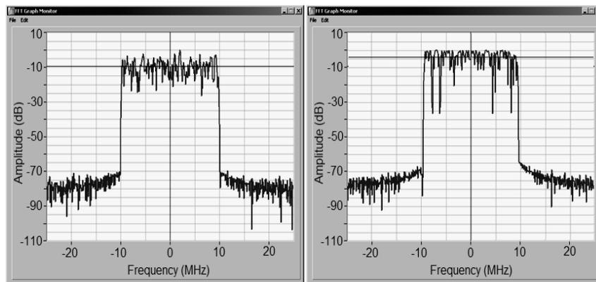
Fig. 2. Frequency spectrum of the test signals: (a) OFDM1; (b) OFDM2.
