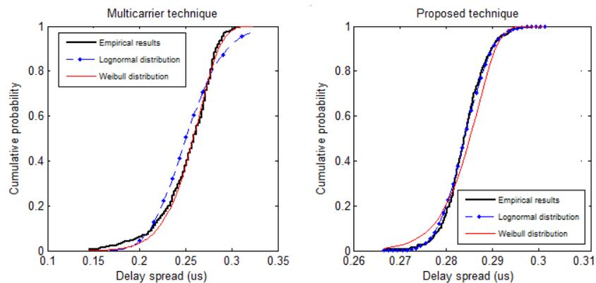
Fig. 7. Cumulative distribution function of r.m.s. delay spread.
