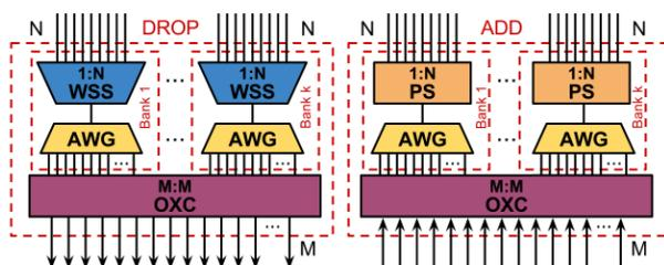
Fig. 6 - A/D structure using 1:N WSS, AWG and OXC.
