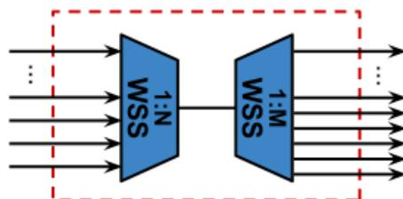
Fig. 3 - Contention N:M WSS using two convention WSS switches.
