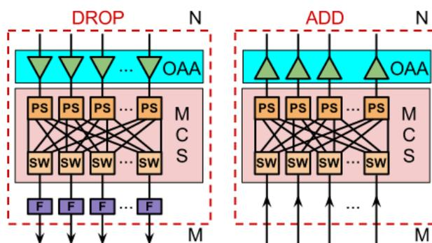
Fig. 4 - A/D structure using MCS, optical amplifiers array and tunable filters.
