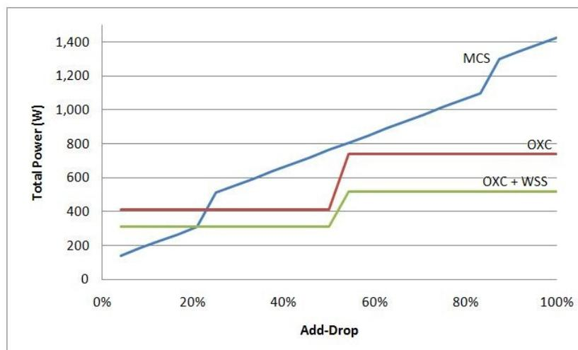
Fig. 8 - Power consumption comparison in a 4-degree ROADM.
