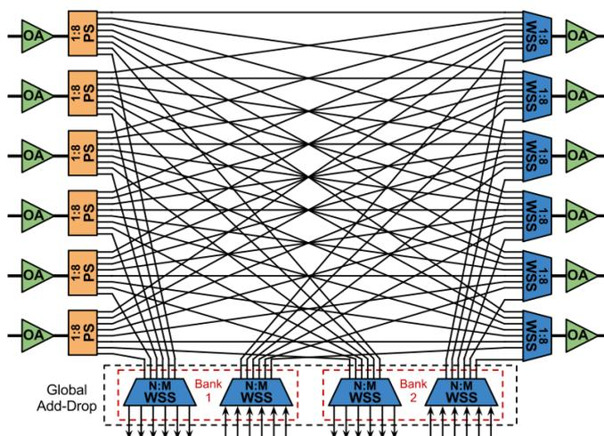
Fig. 2 - Conceptual architecture of NG-ROADM using N:M WSS.
