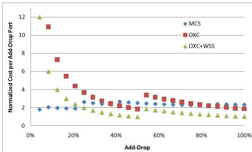
Fig. 7 - Cost per A/D port comparison in a 4-degree ROADM.
