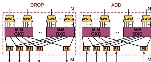
Fig. 5 - A/D structure using M:M OXC, AWGs and PS.
