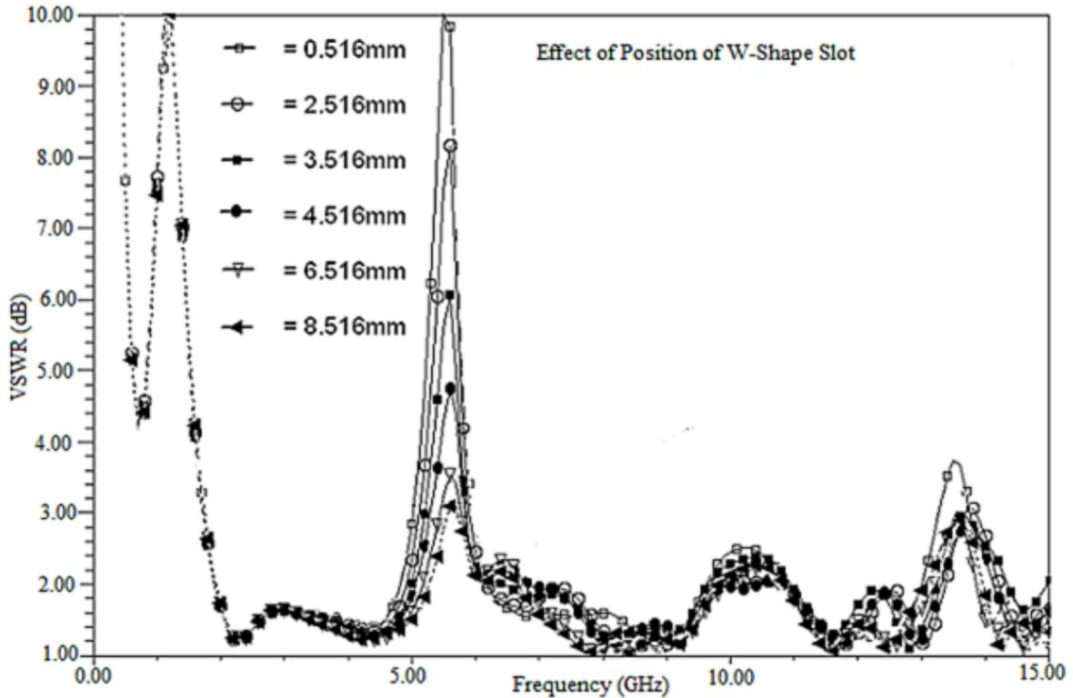
Fig. 6. Simulated results of proposed antenna with respect to various position of slot
