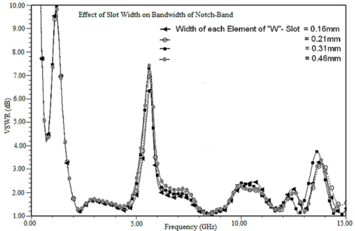
Fig. 5. Simulated results of proposed antenna with respect to various width of slot
